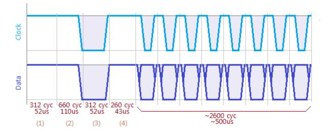
Fig. 3. Byte-level transmission protocol, including (1) and (2) a time to synchronize and allow for client computation; (3) a  $52\mu s$  guard marking the beginning of the byte; (4) a second  $43\mu s$  guard for synchronization; and (5) the 8 bits of the byte.
