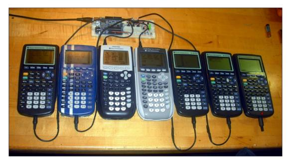
Fig. 1. A seven calculator setup; six of the calculators have been connected to the network.
