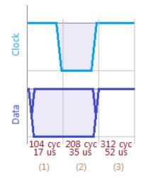
Fig. 4. Bit-level transmission protocol, including (1) a period with the data line set with the bit to transmit and the clock released; (2) a period with the data line set and the clock pulled low; and (3) a period with both the clock and data line released.
